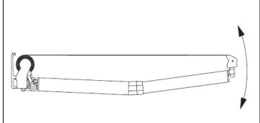
16) To change awning tilt angle loosen (to increase tilt angle) or tighten (to decrease tilt angle) the regulation round head screws in the arm brackets.
