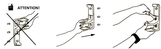
6) Based on the first bracket mark installation places for remaining ones – pay particular attention so that brackets are installed at the same horizontal level and in the same plane.
